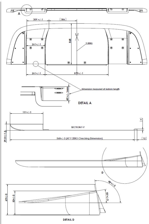
FrontSplitterBrackets' design is free however the front splitter must be rigidly fixed the car's body at least in the area between the vertical projection of the front side members. Outside this area flexible front splitter mountings are allowed. (Certification)
